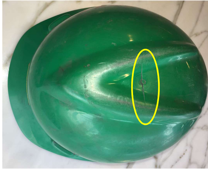
Figure 1 – Cracking in a Green Colored MSA V-Gard Protective Cap
