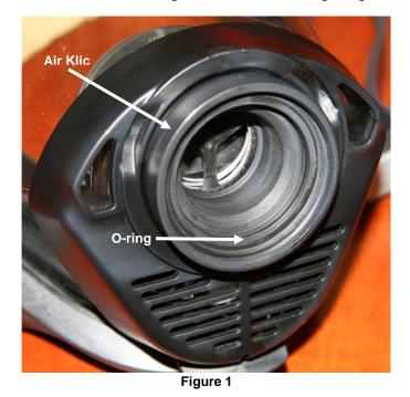
The potential leakage is minimal, amounting to about one minute's worth of air volume using a 30-minute-rated cylinder at a 40 liter per minute breathing rate, <u>and only if the second stage</u> <u>hose is being constantly pulled forward</u>. If the hose is never pulled forward or is only pulled forward intermittently, the leakage would be significantly less. Because of the positive pressure
