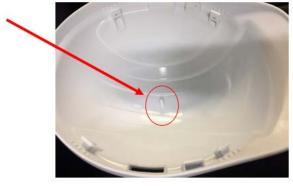
Picture of the sprue vestige inside the hard hat, located at the bottom
